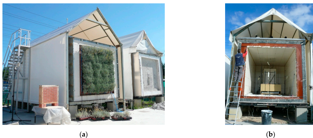
Figure 1. (a) Details of the exterior of the PASLINK test cell: west-facing facade. (b) Interior of the test cell without a sample: south-facing facade.
