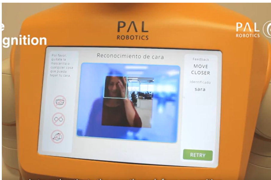
Figure 4.14: The front-end interface of the face recognition functionality on the robot's touchscreen.
