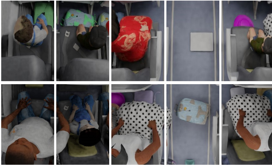
Figure 5.2: Examples of image crops to be processed by multiple DNNs to verify the correct positioning of the luggage for the cabin readiness verification.
