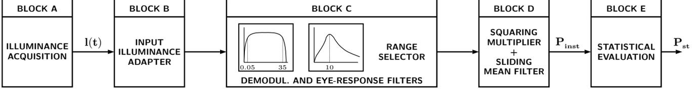
Fig. 2. Block diagram of the adapted illuminance flickermeter.
