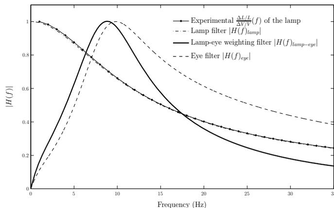
Fig. 4. Frequency response of the filters composing the flickermeter.
