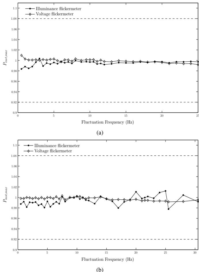
Fig. 5. Test 1 results for sinusoidal (a) and rectangular fluctuations (b).
