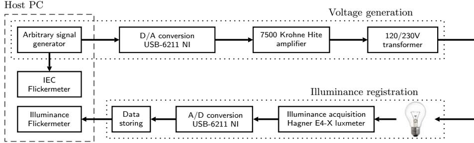
Fig. 3. Scheme of the generation and measurement system.
