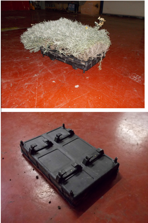
Fig. 3. Recycled polyethylene modules with Helichrysum thianschanicum .
