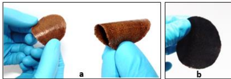
Fig. 6. Composite a) with 75% of OE 12C and 25% of cellulose acetate and b) with 75% of OS 12C , 25% of cellulose acetate and 10% TEC.
