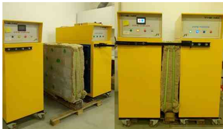
247 Fig. 4. a) Specimen preparation for thermal conductivity test; and, b) Hot box.
