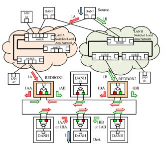
Figure 12. PRP an HSR interconnection by two RedBoxes.
