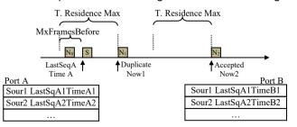
Figure 8. Drop Slider Window. Frames received through port A:  $N_0$  and S. Frames received through port B:  $N_1$  duplicate,  $N_2$  new. If  $N_1$  and  $N_2$  were received through same port A,  $N_1$  would be considered circulating frame.
