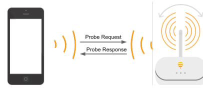
Fig. 1: Device detection based on probe request.
