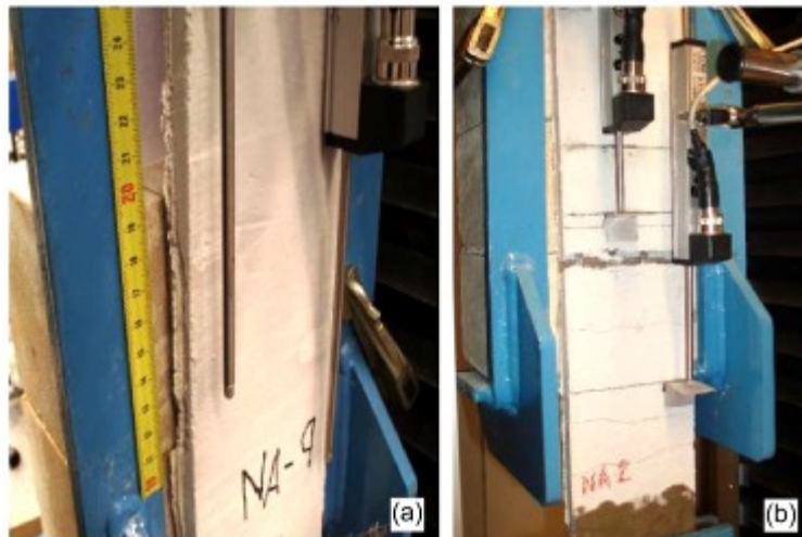
Fig. 12 Failure modes in BTRM specimens: debonding at the substrate-matrix interface in specimens with anchorage length 85 mm (a) and slipping of the fibre rovings from the matrix in specimens with anchorage length 220 mm (b)
