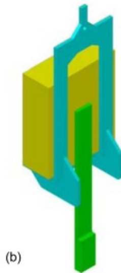
Fig. 7 Single-lap (SL) setup for bond shear tests carried out at UMINHO (a) and TECNALIA (b)
