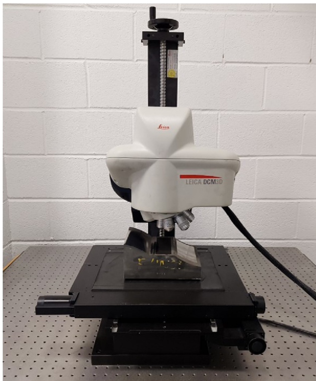
Fig. 7 – Set-up for roughness and topography measurements.
