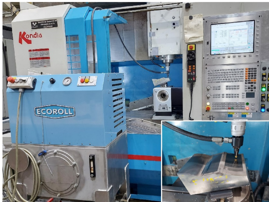
Fig. 2 – 5-axis Kondia HS1000 machining center and Ecoroll Hydraulic pump.
