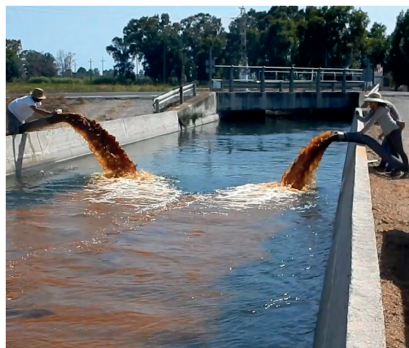
Sediment injection pilot test (IRTA, LIFE Admiclim 2019). Photo: IRTA, Life Ebro-Admiclim ( http://www.lifebroadmiclim.eu/es/ ), with permission
