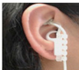
Figure 2. taVNS device. The image shows the electrodes located in the areas innervated by the auricular vagus nerve. Adapted from Warren et al. [59].
