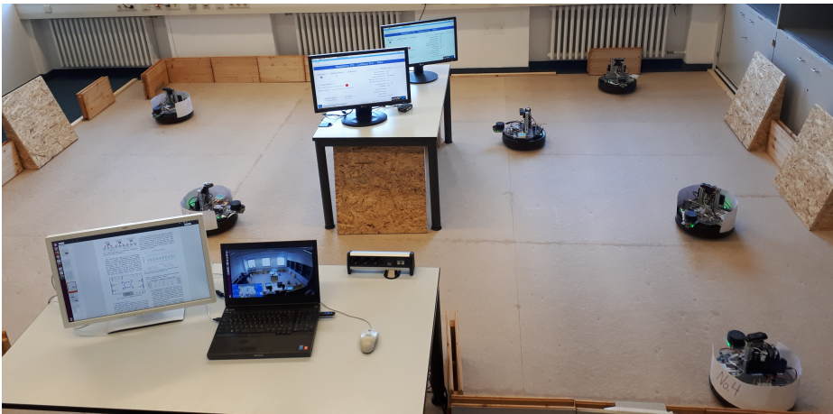
Figure 5.10. Test factory scenario at the Technische Hochschule Nürnberg with up to six ATVs, two machines and a monitoring station.
