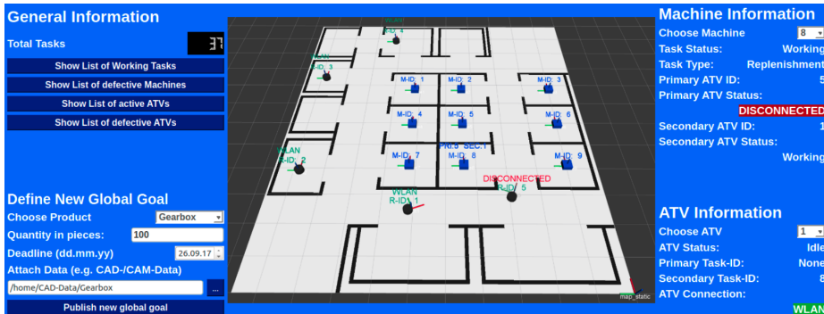
Figure 5.6. Management Panel used for surveillance purposes by visualizing the plant in ROS ( center ) and displaying several information about the plant (top left), the machines (top right) and the ATVs (bottom right). Additionally, it is used to define and publish global production targets (bottom left).
