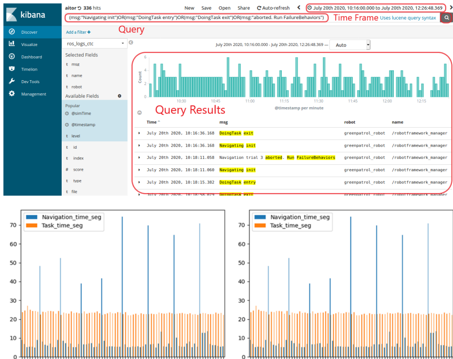
Figure 4.46. Log queries visualized in the elastic search Kibana user interface for the here presented semirandom pest inspection test (up side). The graphs present timing metrics obtained from navigation and inspection tasks during the scouting (down-left side) and spraying (down-right side) plans execution.
