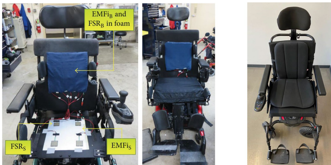
Fig. 5 Example of implementation of FSR sensors on an intelligent wheelchair. On the left, example of sensor implementation under the seat cushion [62]. Right, example of implementation of FSR sensors inside the seat cushion [68]
