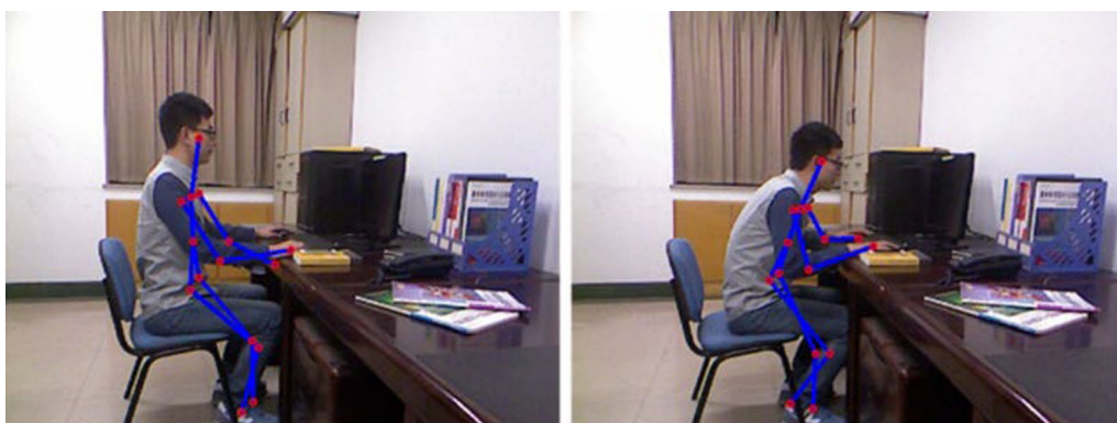
Fig. 3 Example of human body modeling using Kinect camera, presented at [13]. On the left, neutral sitting posture. On the right, frontal tilt of the thorax
