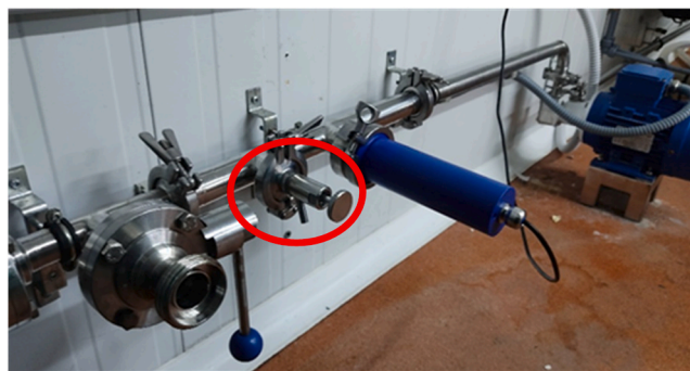
Fig. 1. Measuring and sampling system for milk samples. The NIR sensor (blue cylinder) and the outlet for sampling (indicated with a red circle) are installed in the pipe where the milk flows from the storage tank to the pasteurization system.
