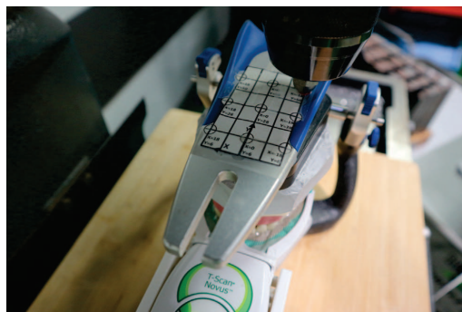
Figure 3. Pattern to control position of input force application point.
