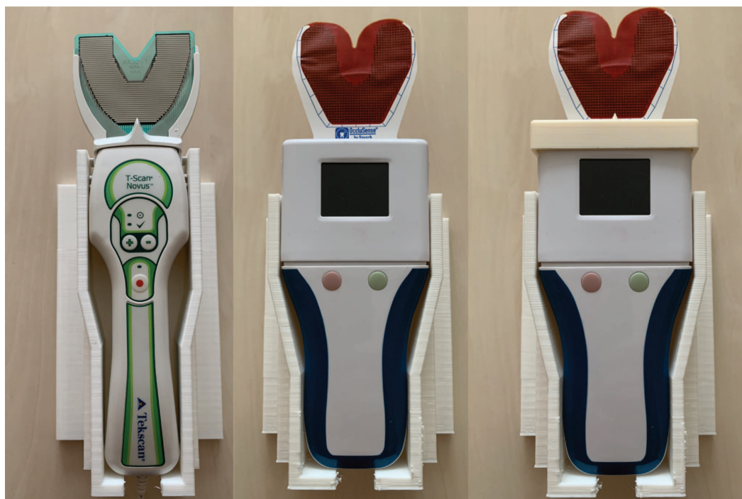
Figure 3. Three digital occlusal analyzer options tested (T-Scan; OccluSense; OccluSense with centering support) with piezoelectric film sensor attached.
