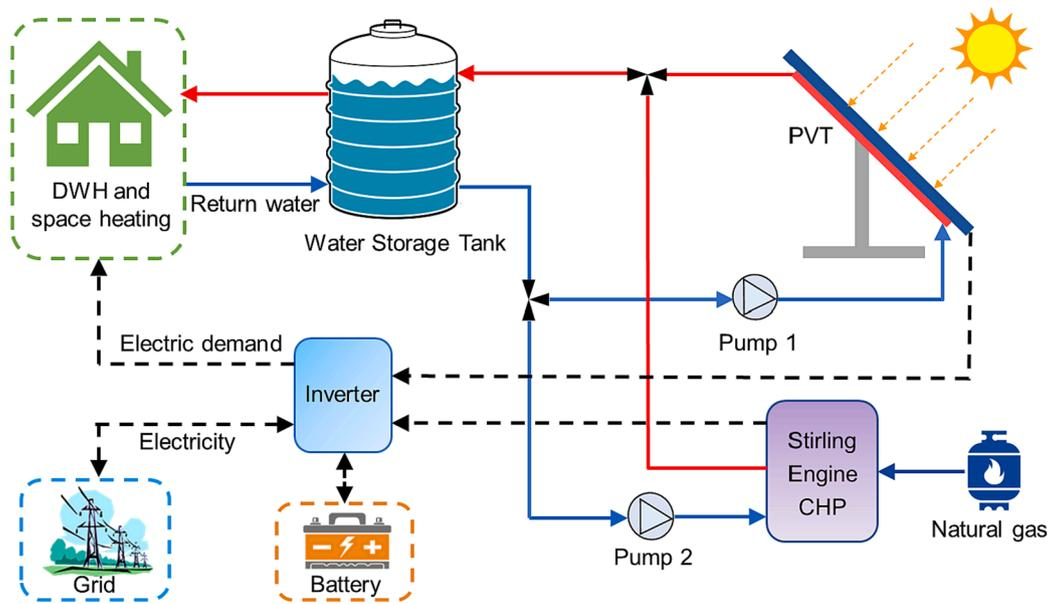
Fig. 1. System topology of PV-T-SE-battery integrated energy system.
