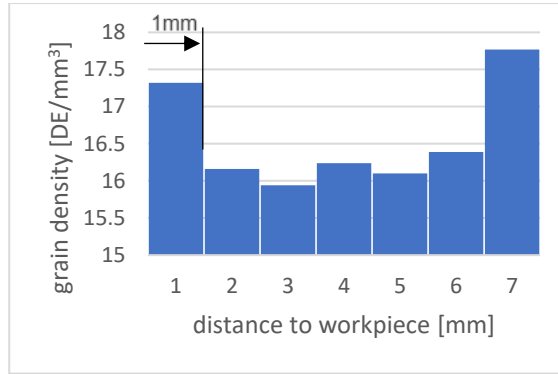
Figure 66. Surface grain density in \mu\text{SM} . Effect of element pile-up from numerical sintering.
