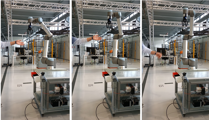
Figure 8.12: Sequence of a non pivoting static collision avoidance (d-APF Controller): The first frame is the initial state of the repulsion, the second frame is a point in between, and the last one represents when the repulsive vector is null because the obstacle is far again.
