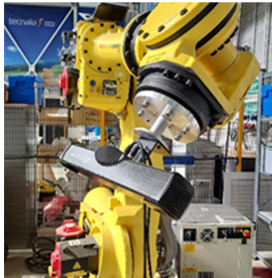
Figure 5. Scanning and robot devices to scan the forged steel flange.
