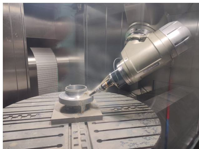
Figure 1. Finished machining of the 5-axis forged flange on ZAYER's Arion G machining center.
