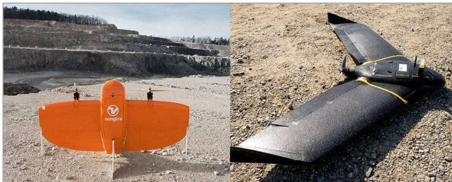
Figura 10. UAV ala fija (WingtraOne / SenseFly eBee X).
