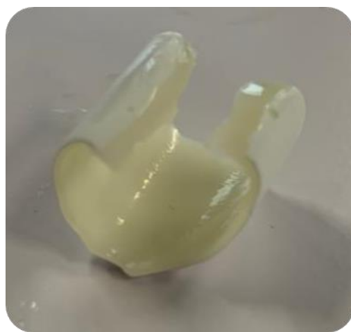
Figure S5-1. Dried film of a blend of PVC-1/PBA and PVC-3/PBA with 25 % of smaller particles in the composition after 5 days drying at 22 °C and 55 % humidity.
