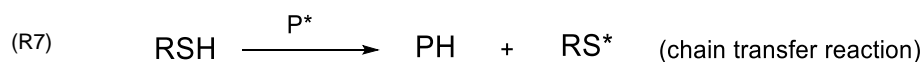
Figure 2.6. Mechanism of grafting reaction in free radical emulsion polymerization of ABS polymer, where I^* is a primary initiator radical or a growing copolymer SAN radical.
