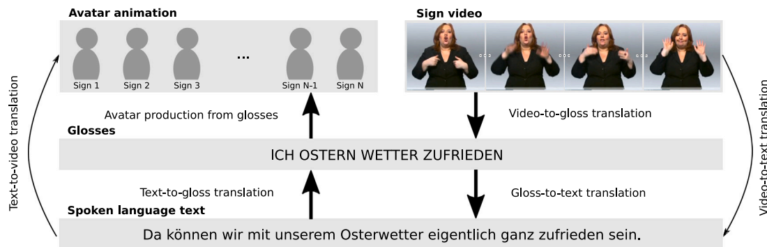
Fig. 1. Video-to-text and text-to-video translation scheme with an optional intermediate step using glosses. The video and the gloss and spoken language translations are sampled from the RWTH-Phoenix-2014T dataset (Camgoz, Hadfield, Koller, Ney, & Bowden, 2018) that contains German spoken language and SL sentences. The translation in English would approximately be “We can actually be very satisfied with our Easter weather”.
