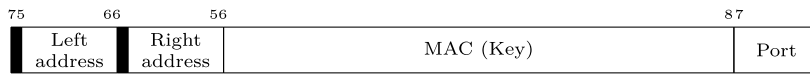
Fig. 4. Data organization in the memory. The length depends on the size of the memory available for the tree and on the number of ports. In this example, the address bus has 9 bits (512 positions) while the port width is 8 bits. Bit 65 tells us whether the right address is real or NULL. Bit 75 does the same for the left address (if the address is negative, it is invalid).
