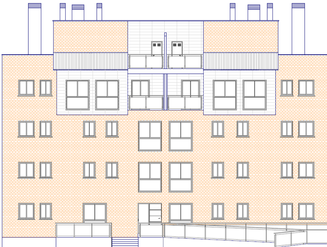
Figure S2. Main elevation of the analysed project with 14 flats of an average of 73.1 m 2 Net Floor Area (NFA) per apartment (minimum NFA of 51 m 2 , maximum NFA of 96 m 2 )
