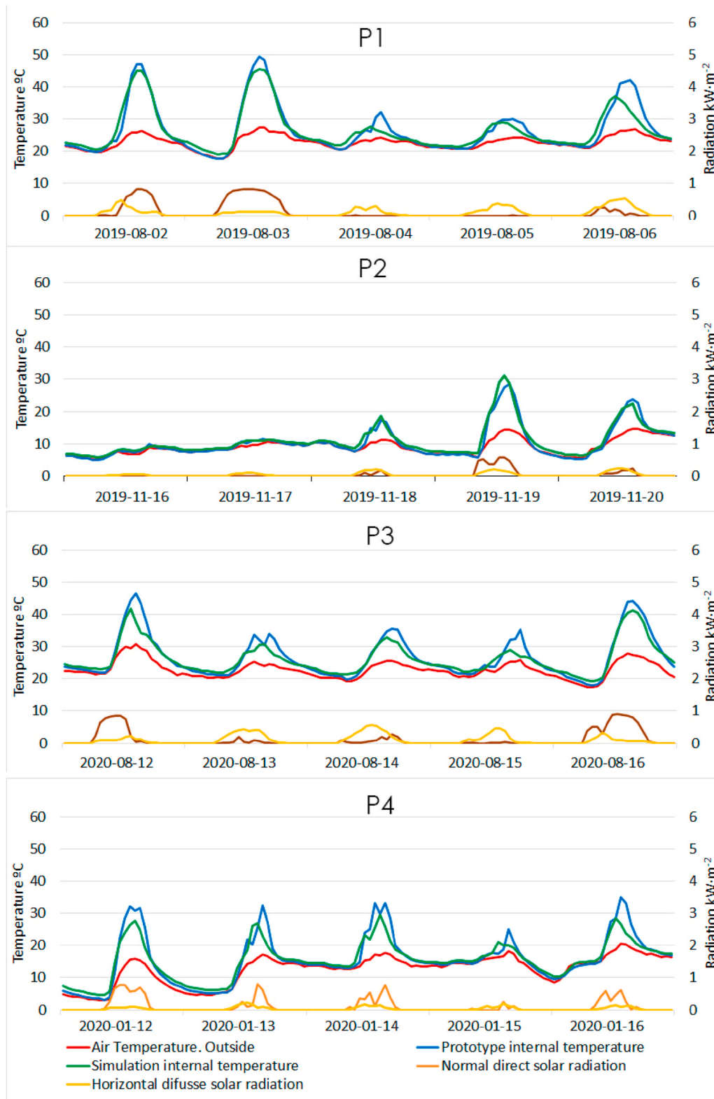
Fig. 9. Comparison of experimental and simulation temperatures in the P1, P2, P3 and P4 periods.
