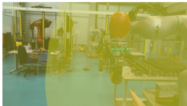
Figure 5. Example view of user perceiving information during the task superimposed on the real scenario. The image shows an example of the information received by the user when inside a hazard zone of yellow level.
