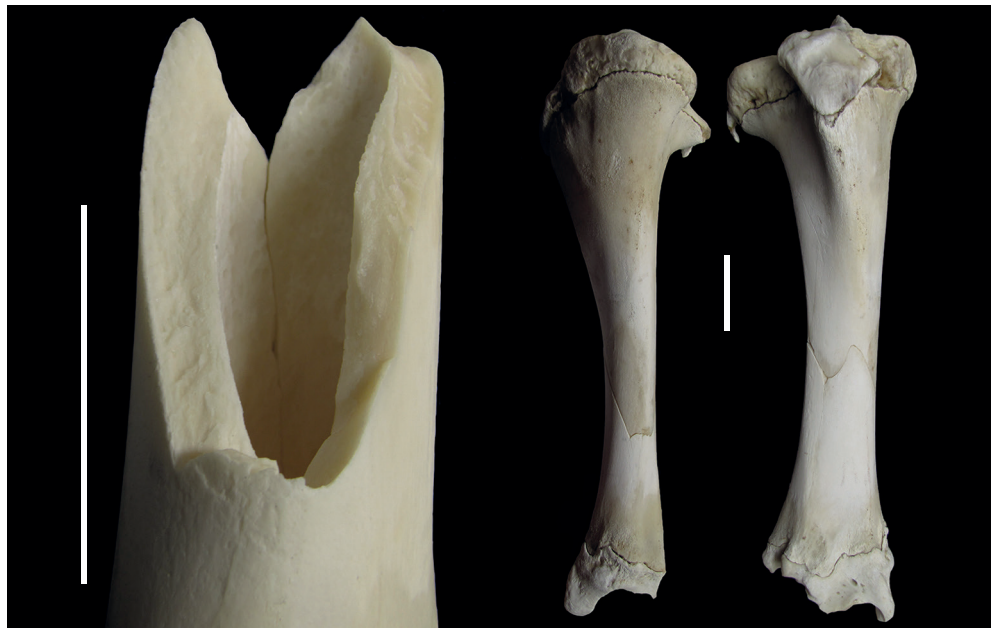
Figure 20 Bos taurus tibia experimentally broken with Bos taurus metapodial; breakage surfaces shows hackle marks indicating dynamic fracture. Scale bar = 5 cm.
