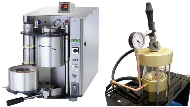
Figure 2.1: Induction melting furnace (left). Arc-melting furnace (right).
