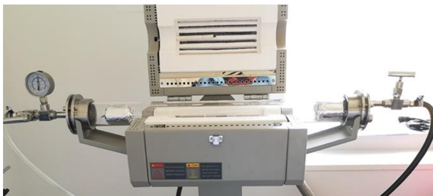
Figure 5.8: Furnace used for the heat treatments with the reflux system installed.
