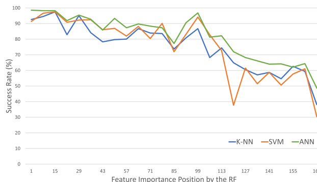
FIGURE 8. Success rate of the K-NN, SVM and ANN based classifiers, with 7 indicators as input selected according to the relative significance provided by the RF approach.
