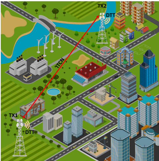
Fig. 1. Representation of an ITCN application combining DTT content transmission and ITCN communications between TX1 and TX2.
