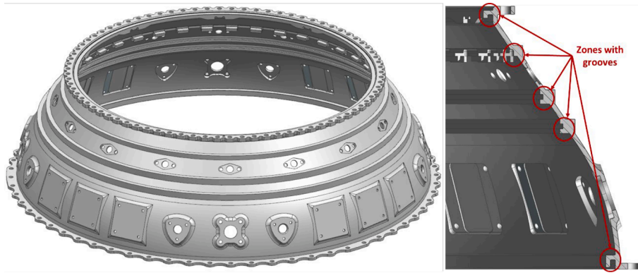
Fig. 1. Aeronautical turbine case and a cutting section view.
