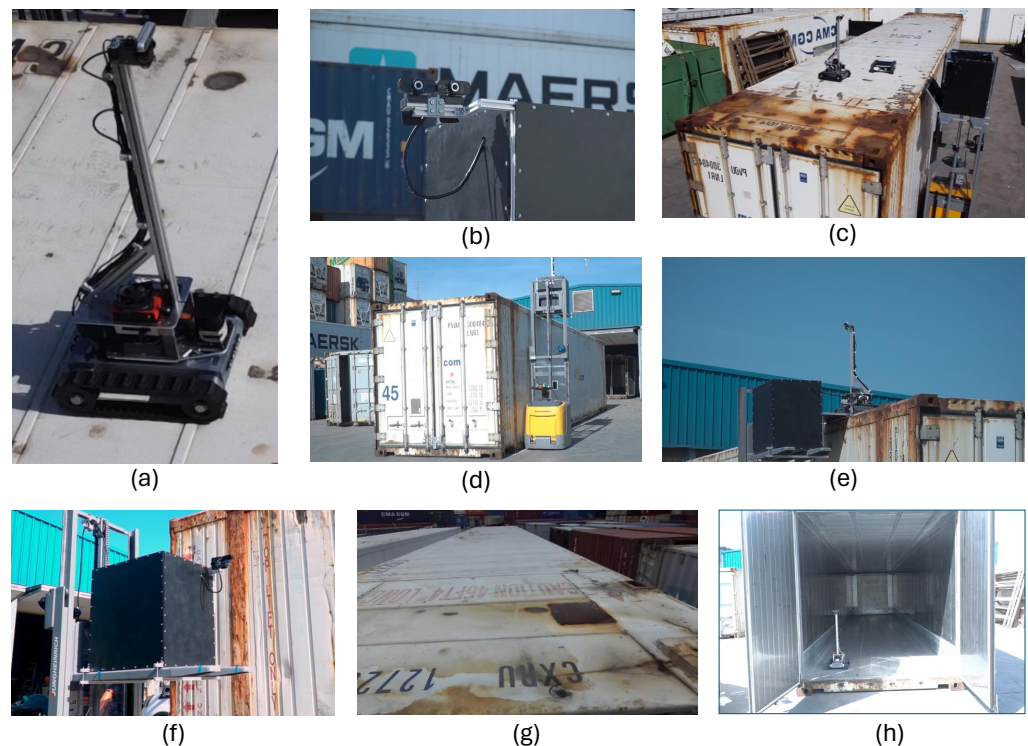
Figure 11. Summary of the field tests conducted for Use Case B: (a) implemented AMR device; (b) vision sensor on board; (c–g) different pictures of the robotic attachment process; (h) image showing that the devised solution can be used to inspect containers from the inside.
