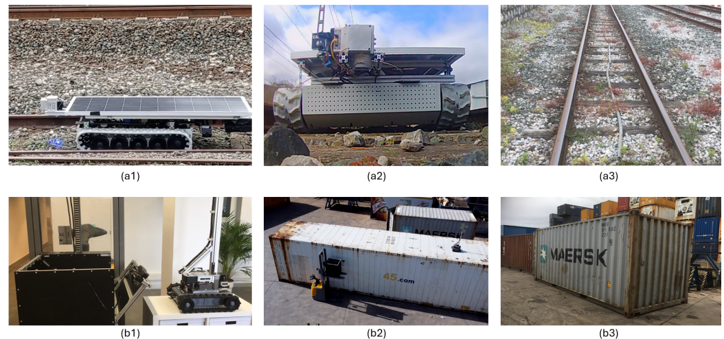
Figure 5. (a1,a2) Rail robot. (a3) Rail testing environment. (b1) Laboratory setup of the top inspection robot and side cameras. (b2) Field test setup in the port. (b3) TEU container for inspection activities.
