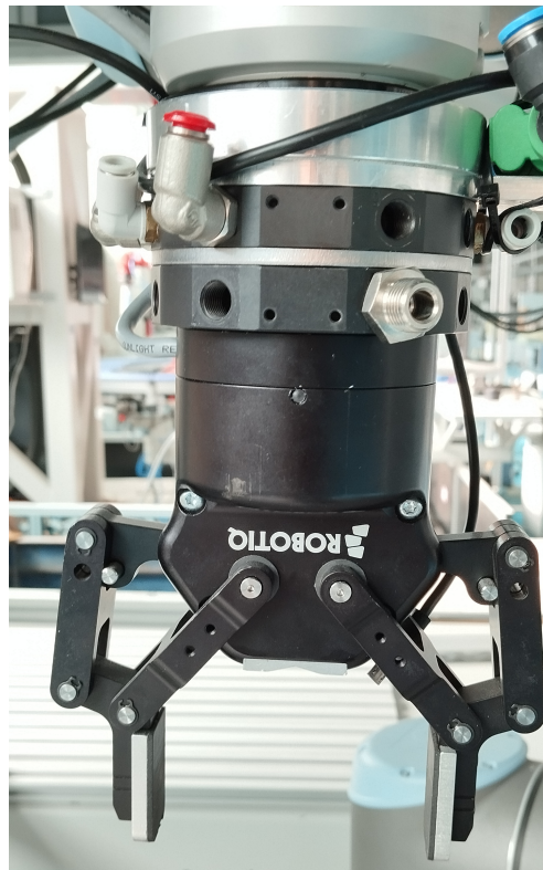
Figure 1.2: Figure showcasing the Robotiq 2f-85. 85 stands for the millimetres between the two pads. This is the gripper used in the project.
