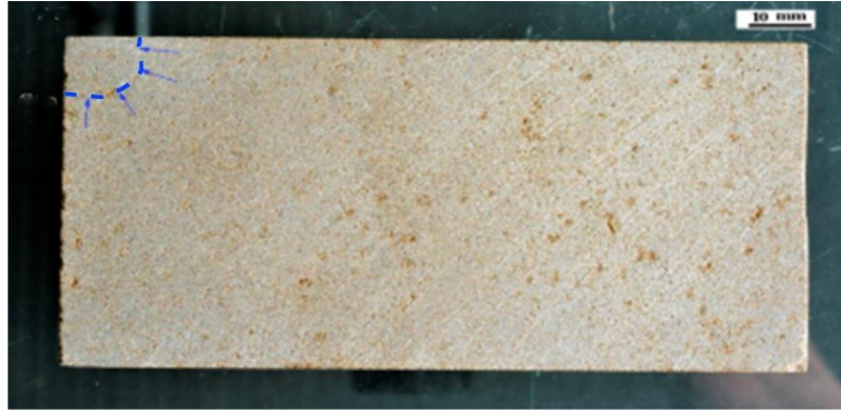
Figure 13. Generated cracks on the A side of the first block after 8 cycles of 5 minutes. The block is rotated 90 degrees.
