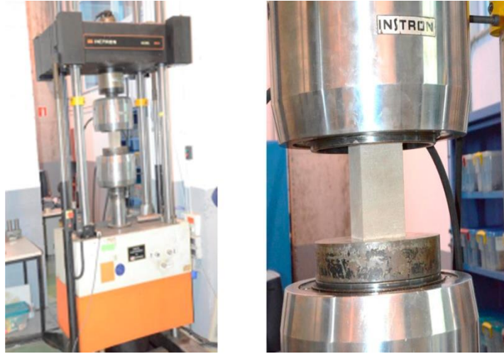
Figure 9. Test process and sandstone block type.
