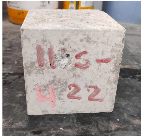
Fig. 5. Specimen of the IIS mix after the cyclic wet-dry aging.
