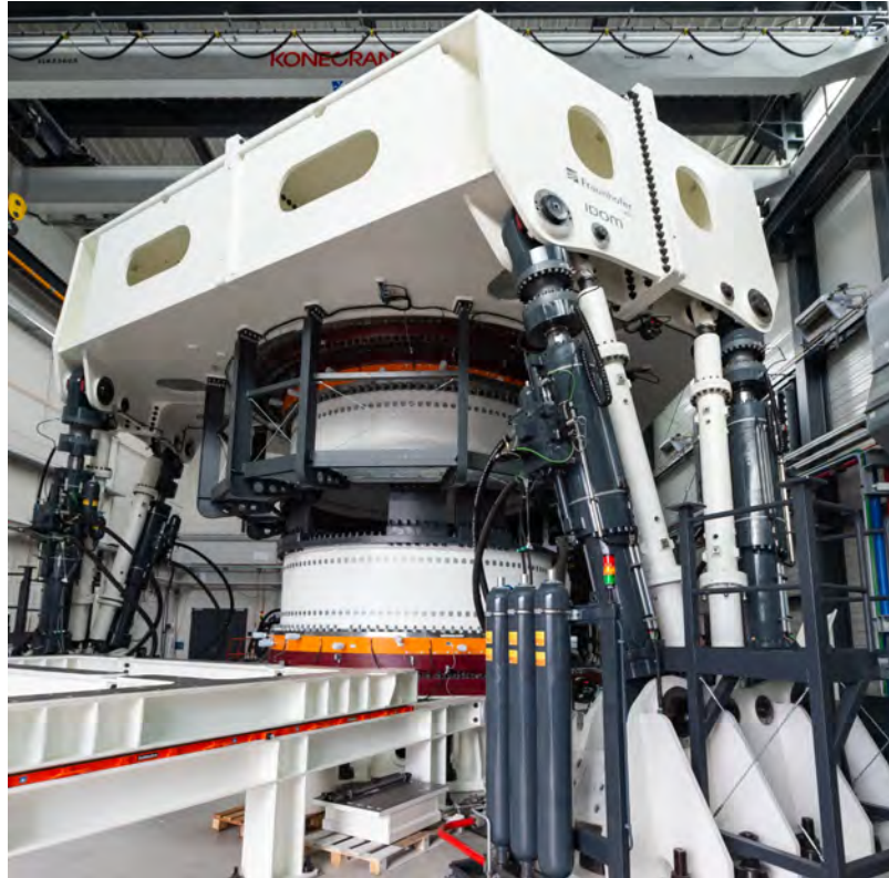
Figure 1.36. IWES BEAT6.1 multi-axial bearing test rig (©Fraunhofer IWES/Ulrich Perrey) [128].
