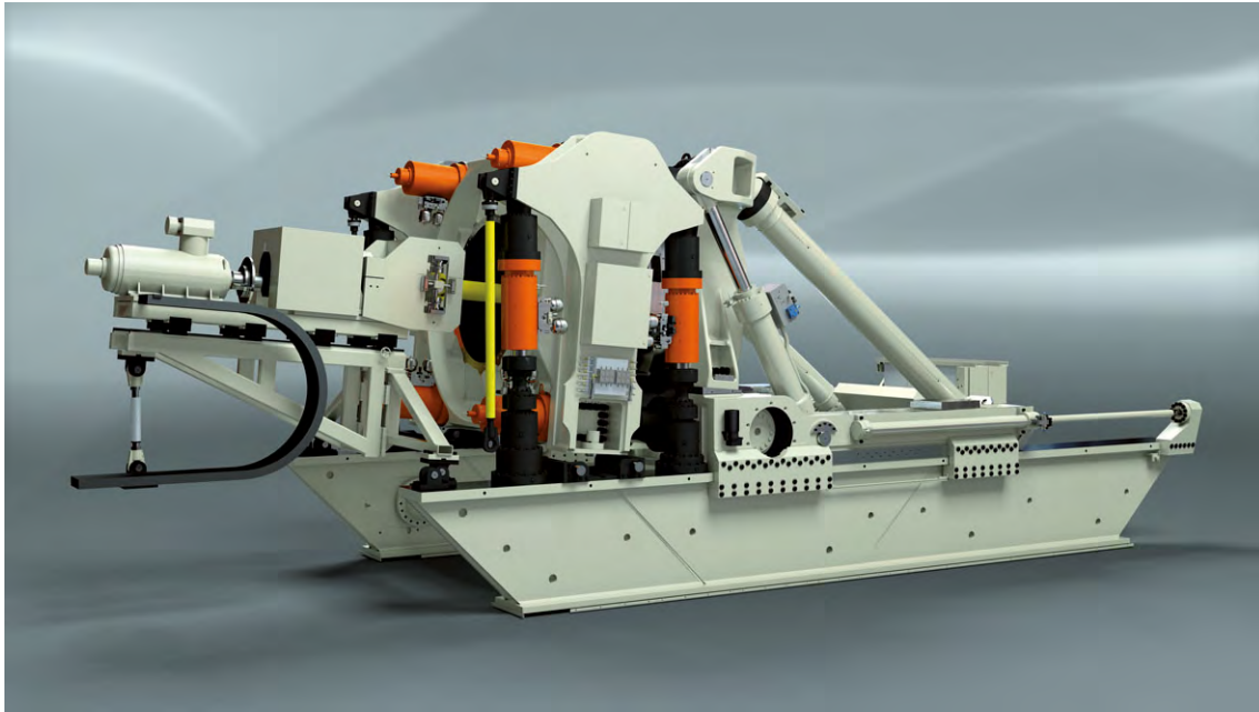
Figure 1.40. “Astraios” test rig from Schaeffler [132].
