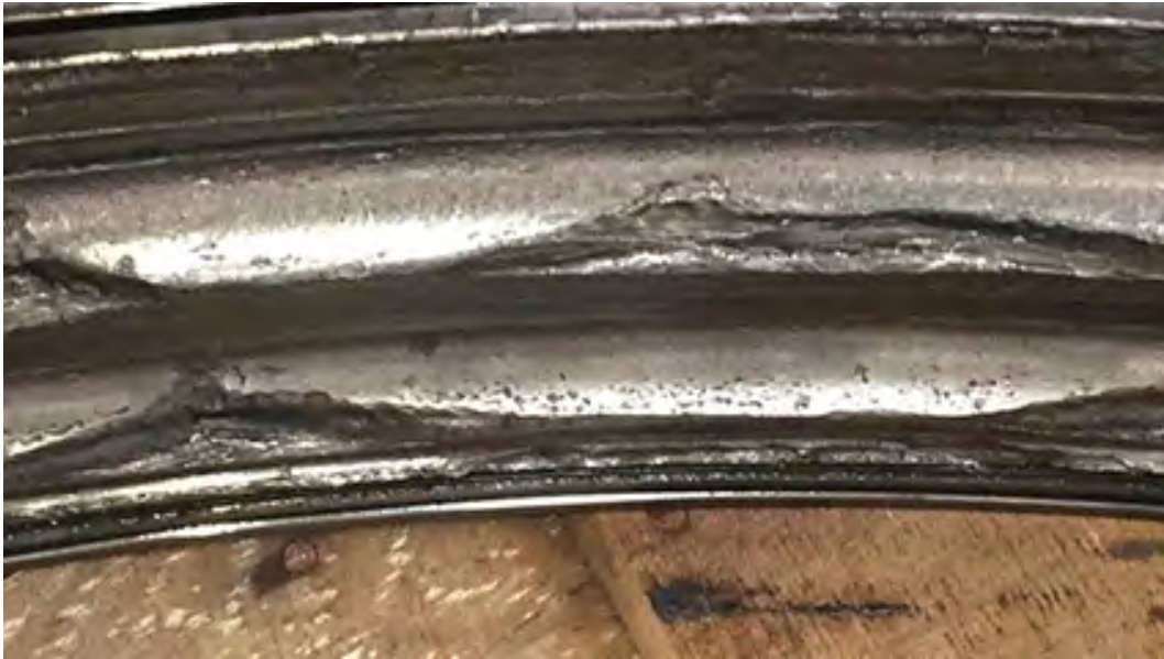
Figure 1.22. Edge loading (contact truncation) failure [43].
