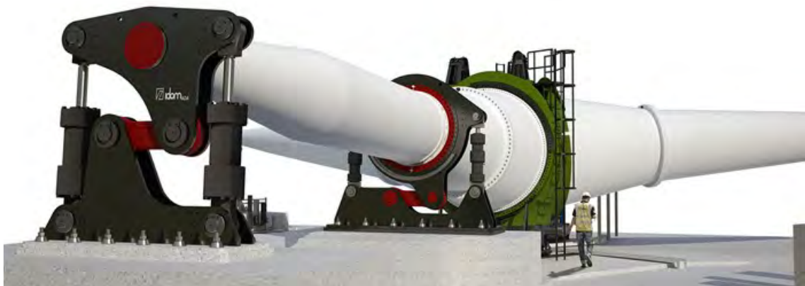
Figure 1.39. WINDBOX test rig [131].
