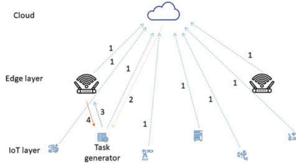
Figure 2: Training procedure of the entire architecture divided in different steps
