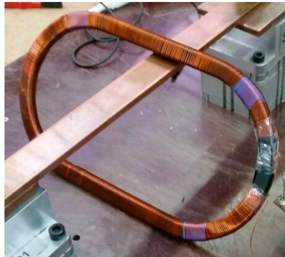
Figure 3. Case study: manufactured non-toroidal CT iron core and secondary winding.
