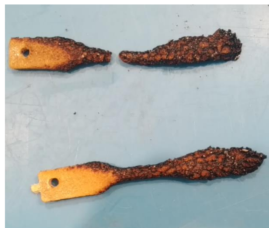
Figure 10. The appearance of specimens after vertical burn test with 30 wt.% of peroxide-treated wool: 30 min peroxide-treated (up) and 24 h peroxide-treated (down).
