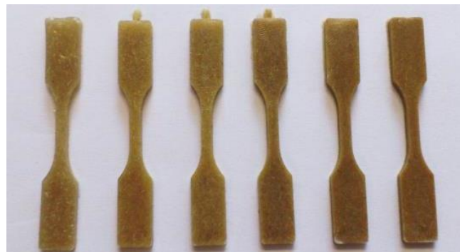
Figure 5. The fiber loading increased from 5 wt.% (left) up to 30 wt.% (right).
