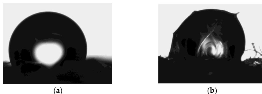
Figure 3. Photographs used for contact angle values measurements: (a) soap-cleaned wool fibers and (b) peroxide-treated fibers for 24 h.
