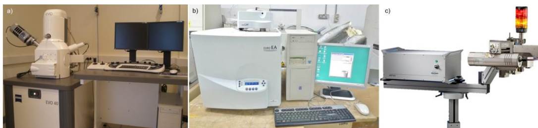
Figure 3.7 (a) EVO®40 SEM-EDS, (b) EuroVector EA-3000 Elemental Analyser, and (c) Artax \mu -ED-XRF. / 3.7 Irudia (a) EVO®40 SEM-EDSa, (b) EuroVector EA-3000 Analizatzaile Elemental, eta (c) Artax \mu -ED-XRFa.
