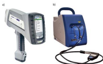
Figure 3.6 Field equipments. (a) \mu -ED-XRF, (b) B&WTEK INC Raman. / 3.6 Irudia Landa-ekipamenduak. (a) \mu -ED-XRF, (b) B&WTEK INC Ramana.
