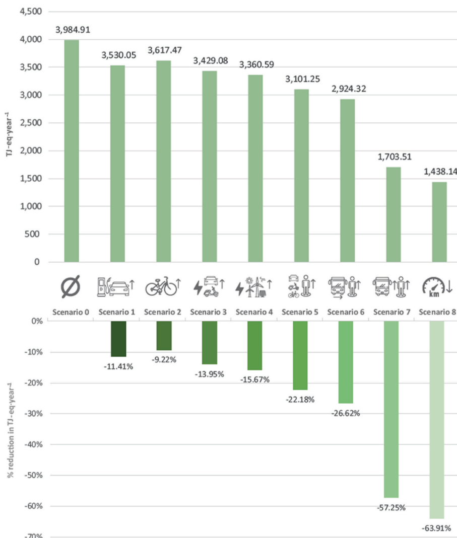
Fig. 6. Comparison of cumulative energy demand in the simulated scenarios.
