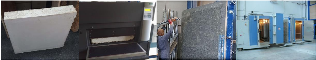
Figure 8: Sample and measurement equipment for thermal conductivity (top and medium left) and wall thermal resistance (top and medium right)
