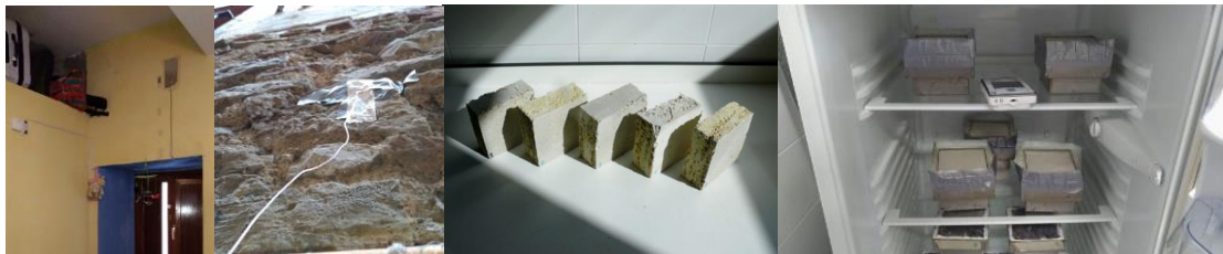
Figure 9: Thermal resistance measurement in situ (left) and samples for testing water vapour transmission properties (right)
