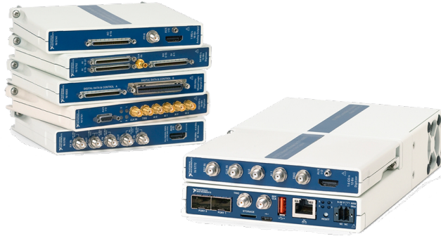
Figure C.8.: FlexRIO device with an IO module mounted and different IO module options.
