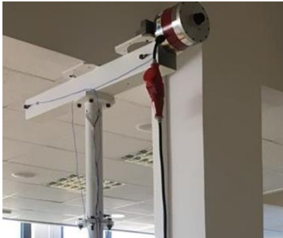
Figure 4-6 Shaker was fixed to the OWT prototype using a screwed steel coupling.
