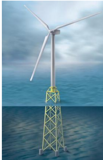
Figure 4-3 Artwork of a jacket-supported OWT [117]
