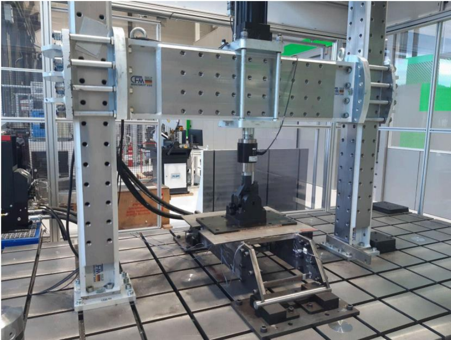
Figure 5-7 Fatigue test machine used in the study case 2.
