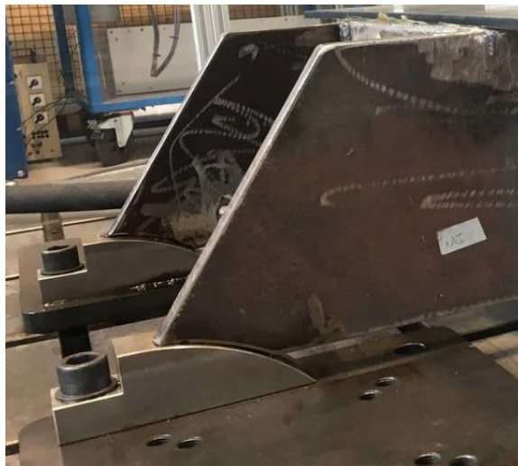
Figure 5-5 Original slot-piece supports.
