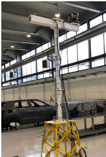
Figure 4-4 Scaled prototype of an OWT used in study case 1.
