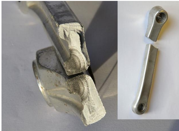
Figure 3-1 Broken steel part due to fatigue. Source: https://commons.wikimedia.org/
