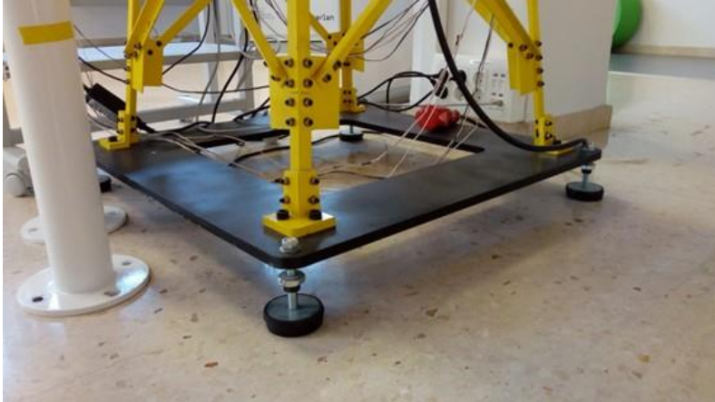
Figure 4-5 Rubber pads on which the OWT prototype rested.
