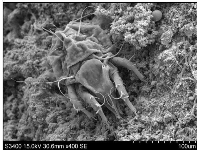
Figure 1.7. Scanning electron micrograph of a “dried” mite invading a biofilter packed with scoria in a biofilter treating toluene.
