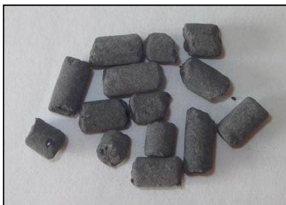
Figure 1.9. ABONLIR™ commercial packing material. The pelletized material is obtained by mixing pig manure and sawdust.
