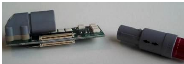
Figure 3.4 – IntFES electronic board and connector of the stimulator cable.
