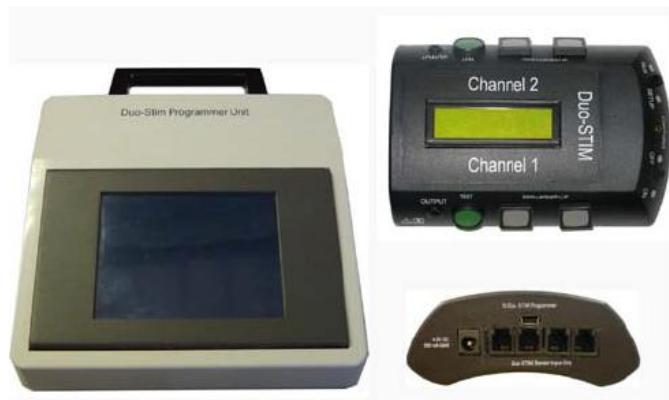
Figure 2.21 – DUO-Stim stimulator device, programmer and portable stimulator units. Reprinted from [43].
