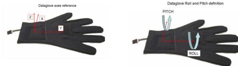
Figure 2.29 – DGTech VHand with reference axes. Reprinted from [77].
