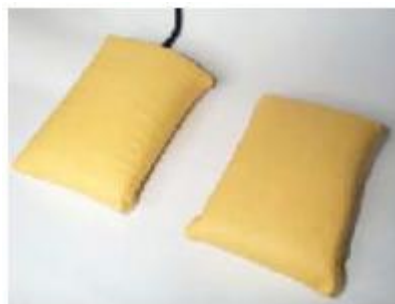
Figure 2.17 – Metal plate electrodes covered by fabric. Reprinted from [40].
