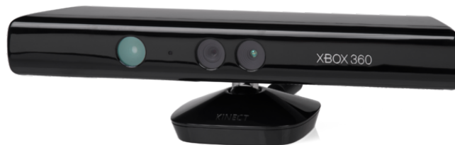
Figure 2.9: The Microsoft Kinect camera. Picture taken by Evan-Amos and distributed under public domain on Wikipedia.
