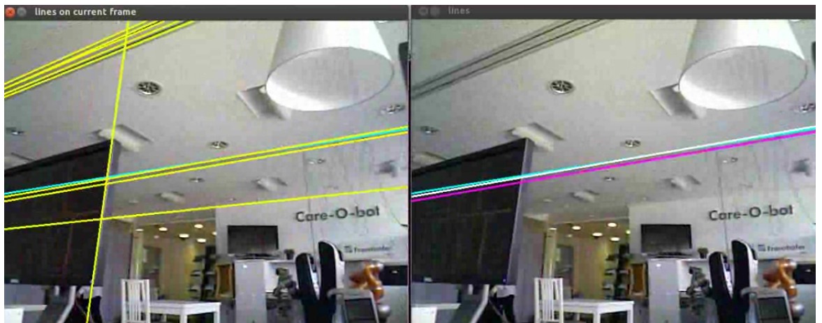
(b) After translating the camera to the left, the projection and the matched line are still correct.
