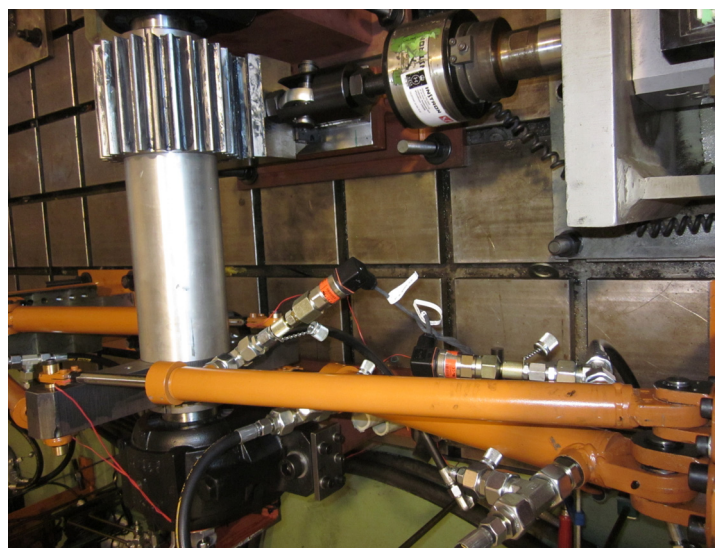
Figure 12. Cylinder chambers pressure transducers.
