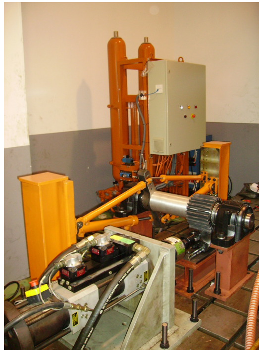
Figure 11. Rack and pinion gear power transmission system.
